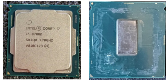
FIG 2: Intel 8700K before and after removing the IHS
